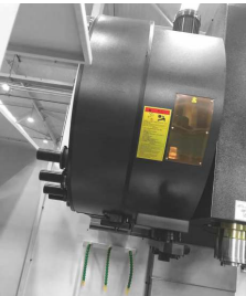
ARM type tool magazine
