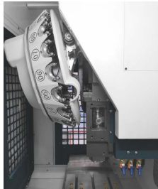
Slant Disc type tool magazine
