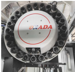
24T ARM type tool magazine
