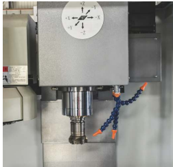
BT40 spindle unit
