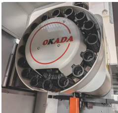
16T ARM type tool magazine
