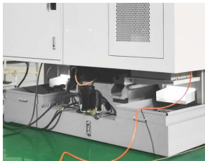
Back-setted chips outlet
