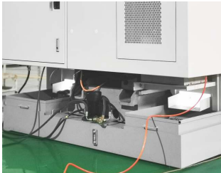
Back-setted chips outlet
