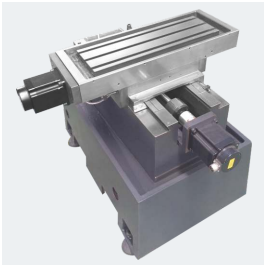
X,Y axes SWALLOW-TAIL shape hard guideway
