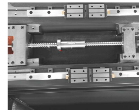
Double nuts ball screw
