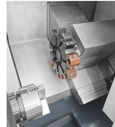
S32T mount chuck+8T servo tool turret
