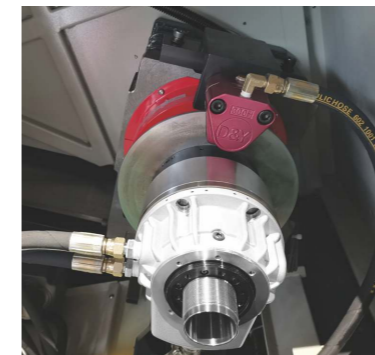
S40M Hydraulic brake and high precision magnet ring encoder
