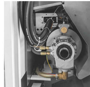
Sub-spindle CS axes and hydraulic brake
