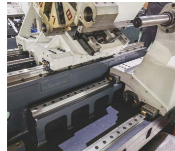
Hydraulic programmable tailstock
